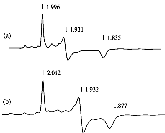
Figure 3. Frozen-glass EPR spectra of complexes generated upon reaction of LMoO 2 (S 2 PPh 2 ) with NBu 4 SH in THF/MeCN: (a) [LMoO 2 (S 2 PPh 2 )] - ; (b) [LMoOS(S 2 PPh 2 )] - .
